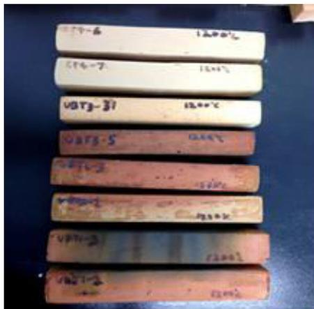
**Figure 3.** Bars fired at 1200°C
