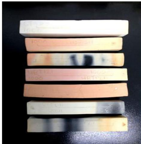
**Figure 1.** Bars fired at 1000° C
