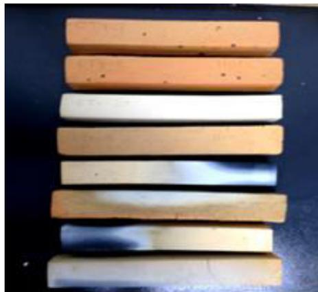
**Figure 2.** Bars fired at 1100°C
