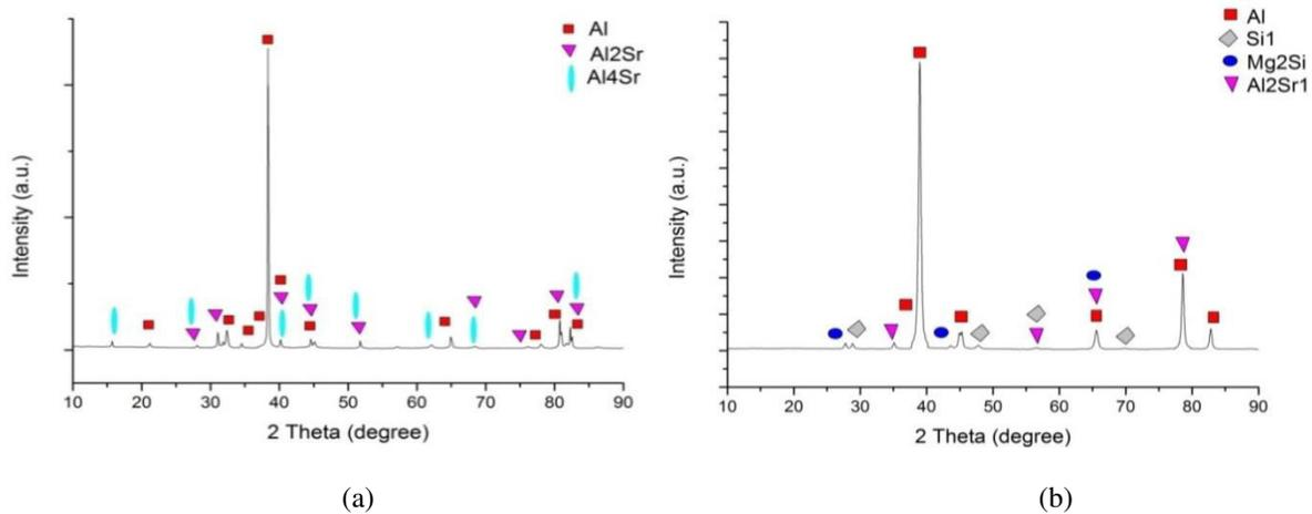
**Figure 3:** XRD analysis of a) Al-10Sr master alloy; b) Conventional cast, Al-6Si-0.97Sr
