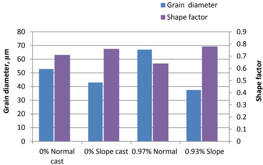
**Figure 2 :** Grain size and shape factor of primary  $\alpha$ -Al for conventional and slope casting
