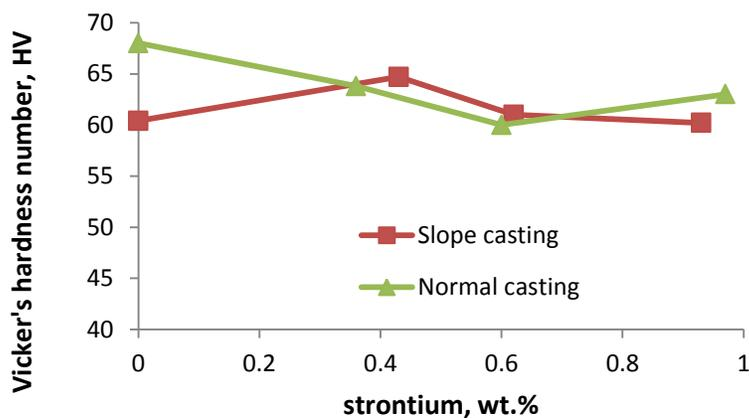
**Figure 4:** Microhardness of conventional and slope cast alloy with variation wt.% of strontium
