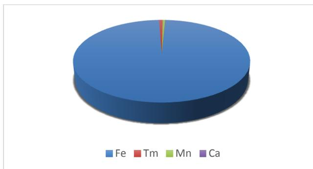
**Figure 1:** XRF analysis of raw mill scales powder.
