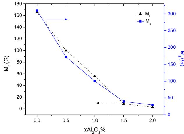
**Figure 4:** The effect of  $M_r$  and  $M_s$  values with variation in  $Al_2O_3$  content.
